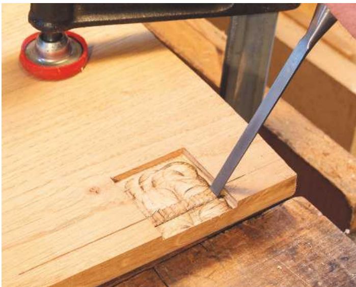
▲ Pic.13 Chopping the knuckle recess, again use the feathering technique
